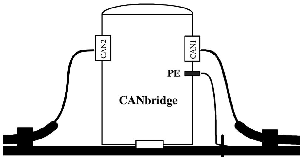
Fig. 7-1: Shield concept CANbridge Industrial DIN-Rail
