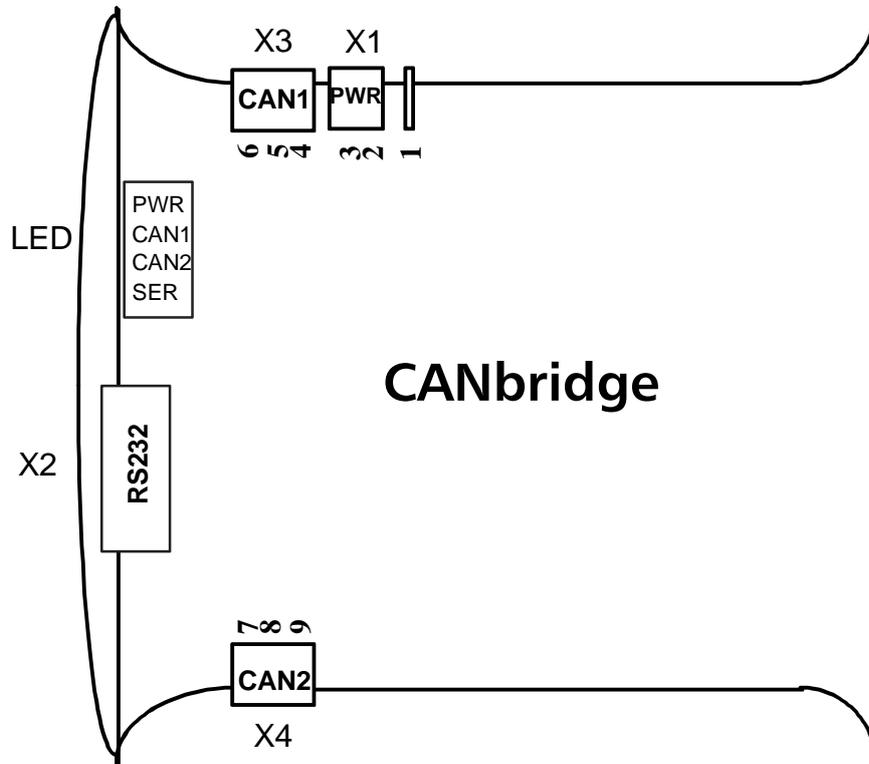
Fig. 3-1: Pin allocation Industrial DIN-Rail version
