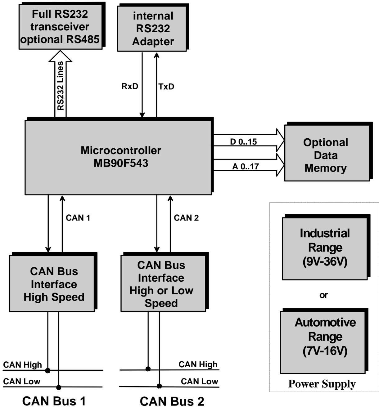
Fig. 1-1: Block circuit diagram CANbridge
