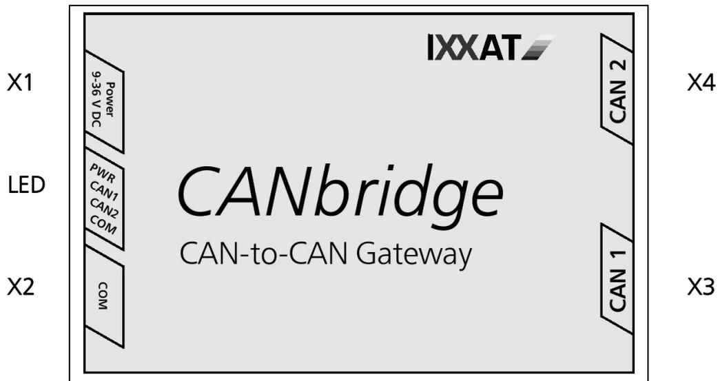
Fig. 2-1: Pin allocation aluminum version
