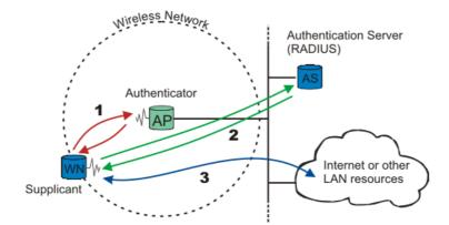
The first step is the physical association between the client and the access point (number 1 on the diagram).
