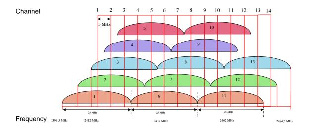
Although the use of "non-overlapping" channels 1, 6, and 11 has limits when products are too close, the 1-6-11 guideline has merit. If transmitter channels are chosen closer than channels 1, 6, and 11 (for example, 1, 4, 7, and 10), overlap between the channels may cause unacceptable degradation of signal quality and throughput.
