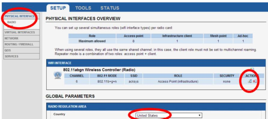
You can select radio interface to set up its Wi-Fi parameters (you can also change IP configuration and services). Set the following essential parameters:
