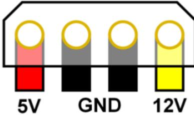
The product can be powered by an ATX 12V power supply (mini 1A)
