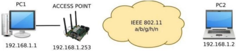
Set up PC2 Wireless network interface according to the default parameters of the ACKSYS AP device (802.11n, channel 6, SSID "acksys", no security).
