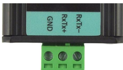
Fig. 4 – terminal on SB485L
