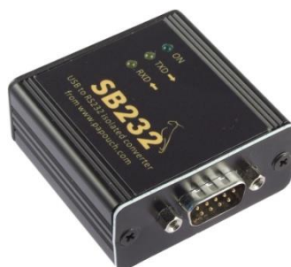
Fig. 22 – Design with RS232 serial line (SB232)
