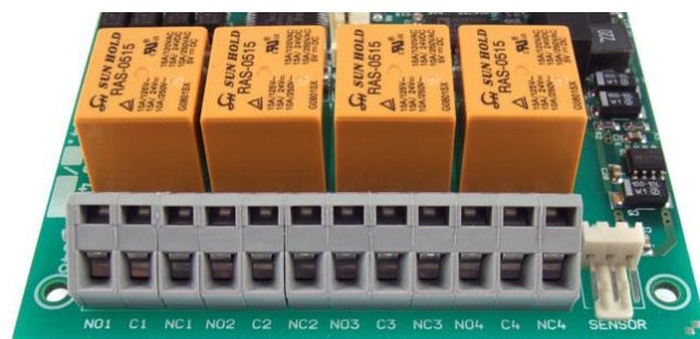
Fig. 7 – make-and-break contacts of output relays
