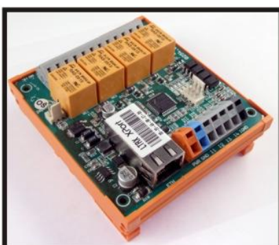
Board with a DIN rail
