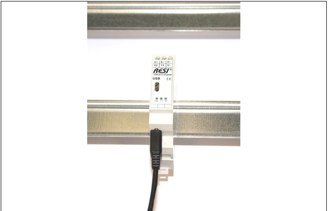
Illustration: Outlet of the USB cable under the 45mm cut-out of a control cabinet to hide the cable under the front cover of the cabinet when connecting components inside the cabinet
