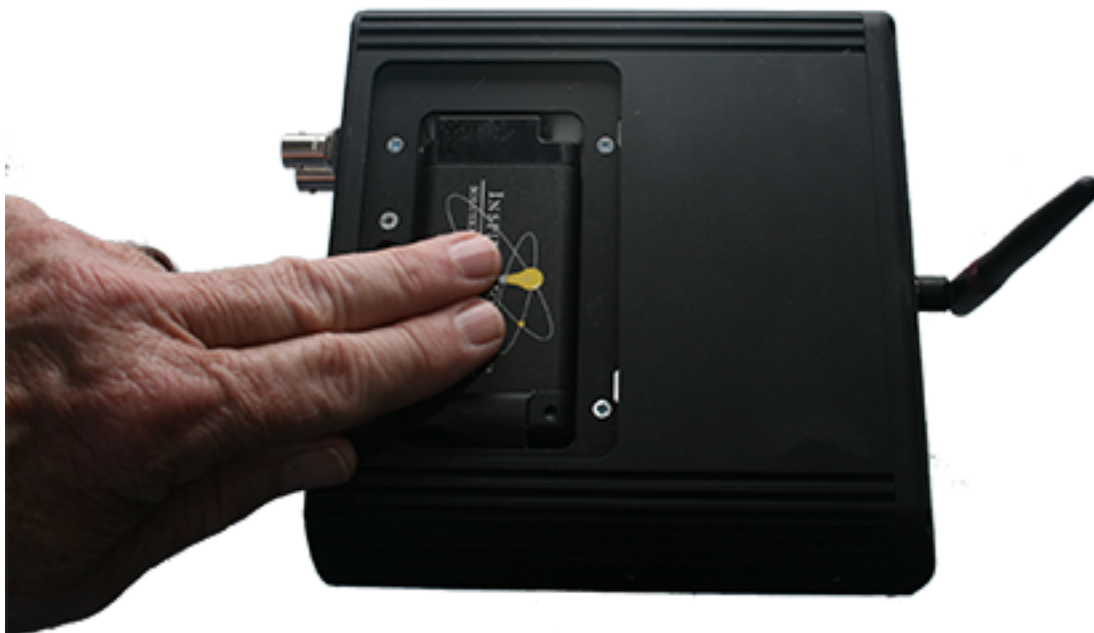
Figure 2.7 - Sodera Battery: Press to Make Contact
