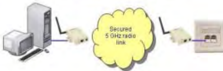
OFFICE NETWORK CABLE REPLACEMENT
