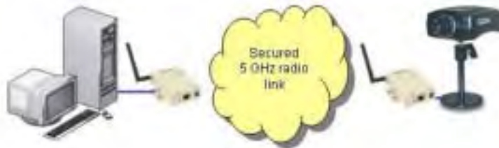
RJ45 ETHERNET CABLE REPLACEMENT BETWEEN TWO EQUIPMENTS
