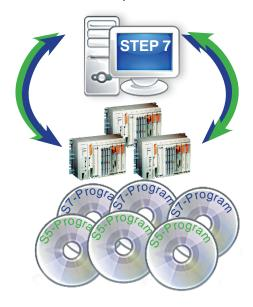
The existing S5 program is completely executable in the X7 CPU.
