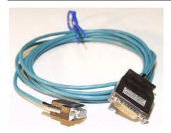
The **COM-Connection PC - SIMATIC S5** connects the PC via the serial interface with the PG-Port of a SIMATIC S5. This programming cable is also suitable to connect terraLink and S5 (null modem needed).
