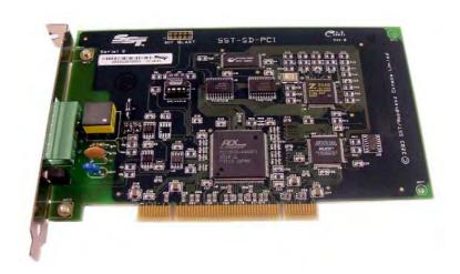
The SST Data Highway Plus interface card can connect your PCI bus computer to Allen-Bradley Data Highway Plus (DH+) and 1771 Remote I/O (RIO) (adapter or scanner mode) networks ▲
