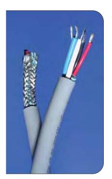
Bulk Tray-Rated, 600V-rate DeviceNet trunk cable is designed for use in Class I cabling installations. In such installations this cable can be routed adjacent to other 600 V or Class I rated cables in order to eliminate the use of conduit by "laying" this cable in a cable tray. Temporary field installations can be completed to the trunk by attaching Mini-Change® field attachable connector.
