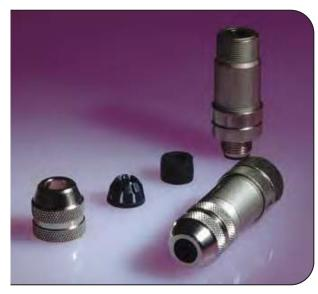
Profibus Micro-Change® field-attachable connectors allow you to make field connections to bulk cable. The screw terminations allow for simple field installation of the data line which can then be connected to a product such as an active I/O module.
