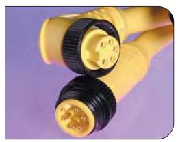
Both single- and double-ended 5P Mini-Change® cordsets, receptacles and tees are used to connect power to a variety of devices including active I/O modules. Female connections bring power safely to the blocks. When powering active modules the molded Mini-Change connector end of the cable connects to the block while the flying lead end is connected to the power supply output. Double-ended cordsets are used to provide a quick-disconnect on the power source.
