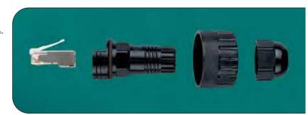
advance the exact length between each connection point. The RJ-Lnxx® field attachable connector enables bulk cable to be pulled to the exact required length, and then terminated to the RJ-45 plug using readily available crimp tools. The completed assembly provides the same sealed, robust connector as the RJ-Lnxx overmolded cordset.
