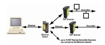
The SST Remote DeviceNet Scanner controls I/O devices connected to a DeviceNet network without the need of a local PC. DIN rail mountable, up to 16 SST Remote DeviceNet Scanners can be connected to one Ethernet switch which is then connected back to a PC residing on an Ethernet network. The PC allows users to remotely access diagnostic information on the SST Remote DeviceNet Scanner and the DeviceNet network.
