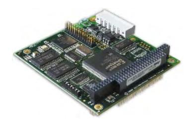
The SST DeviceNet Generation III (DN3) PC/104 interface card can connect your PC/104 bus computer to DeviceNet networks▲
