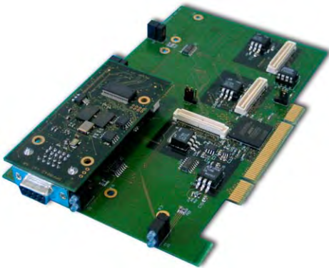
Test and evaluation board, carries up to 4 ENI modules
