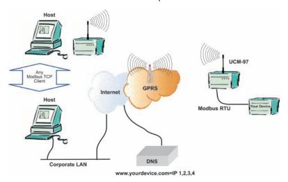
multiple ModbusTCP clients. When using the UCM-97 as a Wireless ModbusTCP to Serial ModbusRTU device, it can be commissioned to operate either on the public Internet with
