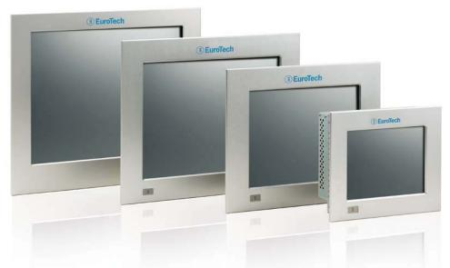
All the **MTXX** family of monitors have high brightness TFT displays, wide viewing angle and long life rear lamps (50.000 hours at 25°C), they are all extremely compact and come in a wide range of sizes. They can be connected to an external computer, such as our Box Computers, using a standard VGA cable. The touch-screen version provides both RS232 and USB interfaces.
