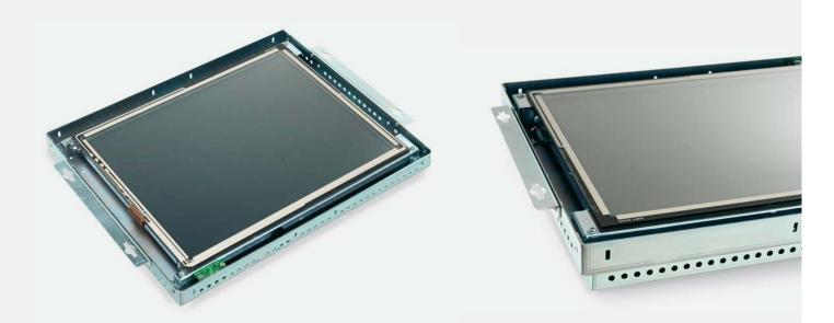
All the **OFXX** family of monitors have high brightness TFT displays, wide viewing angle and long life rear lamps (50.000 hours at 25° C), they are extremely compact and a come in a wide range of sizes. They can be connected with an external computer, as our Box Computers with a VGA standard cable. The touch screen version provides both RS-232 and USB interfaces. This family is particularly indicated for rear panel mounting solutions.
