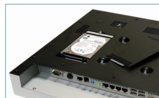
6. Slim HDD bay design for easy service.
