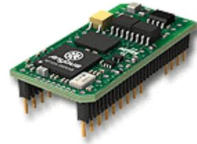
The New Anybus-IC is a complete DeviceNet slave interface on a 32 pin dual in-line housing. It can be inserted into a host product with only a 5 volt 85mA power supply, and a DeviceNet connector required to achieve instant connection to the DeviceNet network.
