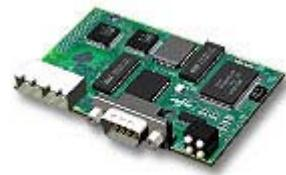
The Anybus-M AS-Interface Master module supports up to 62 slaves with a maximum of 248 digital input, 186 output signals and 124 analog values.
