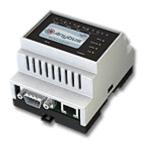
Anybus RemoteCom Ethernet / Web version enables remote management of industrial devices and machinery from a standard web browser. RemoteCom is an easy-to-use web gateway which acts as a Modbus bridge and gives remote access and control of serial devices over Ethernet, Internet, LANs, and telephone modems
