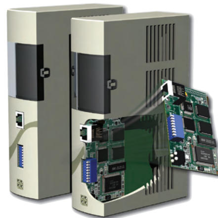
Example of a motion controller using Anybus-S Ethernet as its communication card
