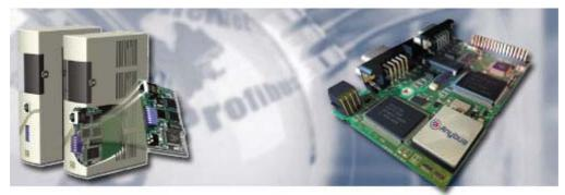
Drive Profile technology encorporated into the proven Anybus-S concept extends the software functionality and makes it easier for drive manufacturers to make their products comply to the latest communication standards for drives. The Anybus module does not only contain the complete profile, it is also fitted with an application interface that is the same irrespective of what fieldbus is used.
