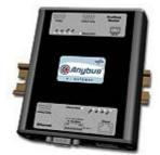
The Anybus X-gateway copies I/O-data in both directions thus enabling an exchange of data between the two networks. Default I/O configuration is 20 bytes Input and 20 bytes Output. Changing default settings is very simple and is carried out using the RS232 configuration port and a standard terminal interface on a PC, such as Hyper Terminal for Windows.
