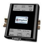
The Anybus X-gateway copies I/O-data in both directions thus enabling data exchange between the two networks. Default I/O configuration is 20 bytes Input and 20 bytes Output. Changing default settings is very simple and is carried out using the RS232 configuration port and a standard terminal interface on a PC, such as Hyper Terminal for Windows. The Anybus-M AS-Interface Master module supports
