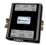
The Anybus X-gateway copies I/O-data in both directions thus enabling data exchange between the two networks. Default I/O configuration is 20 bytes Input and 20 bytes Output. Changing default settings is very simple and is carried out using the RS232 configuration port and a standard terminal interface on a PC, such as Hyper Terminal for Windows.
