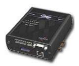
The Anybus X-gateway makes it possible to transfer data between DeviceNet network up to an Ethernet network which can be Modbus TCP/ EtherNet/IP or HTTP. The gateway also features CIP message routing between Ethenet/IP and DeviceNet.
