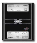
The Anybus X-gateway copies I/O-data in both directions thus enabling data exchange between the two networks. Default I/O configuration is 20 bytes Input and 20 bytes Output. Changing default settings is very simple and is carried out using the RS232 configuration port and a standard terminal interface on a PC, such as Hyper Terminal for Windows.
