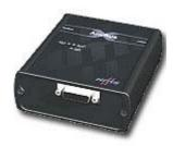
The Anybus X-gateway J1939 Gateway provides connectivity between a Modbus RTU (serial) network and a J1939 Heavy Duty vehicle (CAN) network. The ABX appears as a Modbus Slave device allowing a Modbus Master to read or write data from the J1939 network.
