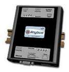
The Anybus X-gateway copies I/O-data in both directions thus enabling data exchange between the two networks. Default I/O configuration is 20 bytes Input and 20 bytes Output. Changing default settings is very simple and is carried out using the RS232 configuration port and a standard terminal interface on a PC, such as Hyper Terminal for Windows.
