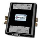
The Anybus X-gateway copies I/O-data in both directions thus enabling data exchange between the two networks. Default I/O configuration is 20 bytes Input and 20 bytes Output. Changing default settings is very simple and is carried out using the RS232 configuration port and a standard terminal interface on a PC, such as Hyper Terminal for Windows.
