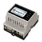
The Anybus Serial Server is an Ethernet Virtual COMport to RS232 and RS485 COM-port gateway. Together with a special software driver in a PC, it can be used as a remote serial port. PC applications designed to access data using normal serial COM-ports, can access the data through the remote Anybus serial server without any software modifications. The LAN/Internet network together with the serial server and driver can be viewed as a long "virtual" serial cable.
