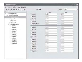
For time-dependent events, such as the SYNC telegram in the case of CANopen, up to 11 timers (CAN 300) or 16 timers (CAN 400) are available in the CAN modules up to a resolution of 1ms. Each timer can transmit any CAN telegram. The timers can be started, stopped, and changed from the PLC.
