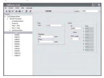
CAN telegrams can be transmitted or timers started via freely programmable scripts on certain events such as "Power ON" or "PLC Stop -> Run".
