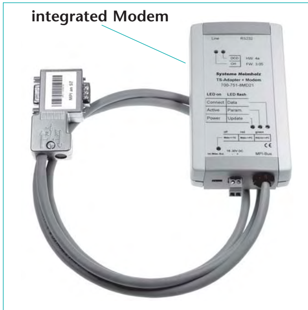
SSW7-TS with integrated modem; analog/ISDN
