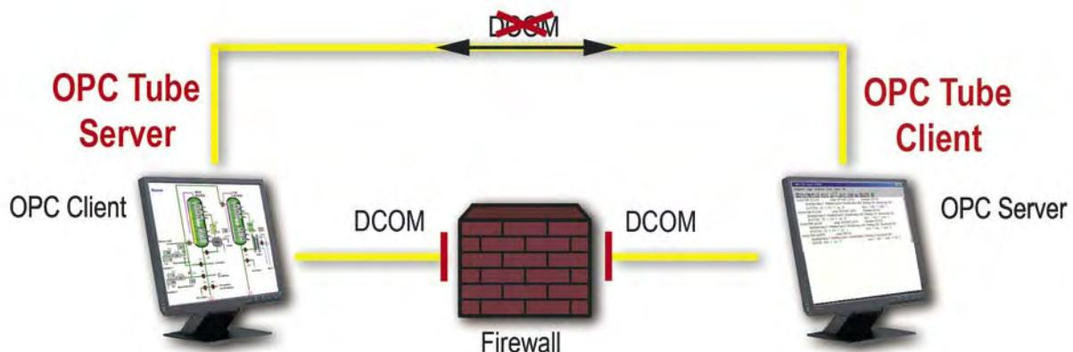
OPC Tube enables OPC communication between distributed computers without DCOM configuration
