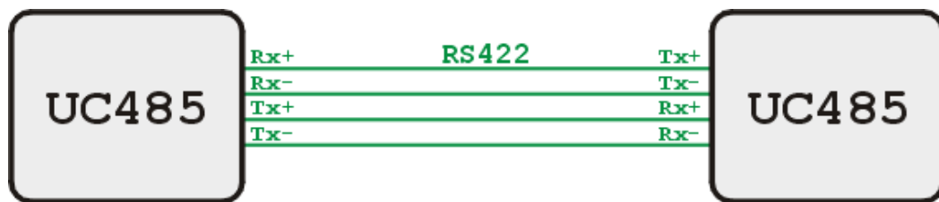
Fig. 13 – An example of a system with an RS422 line interconnection. Termination is connected in both modules.
