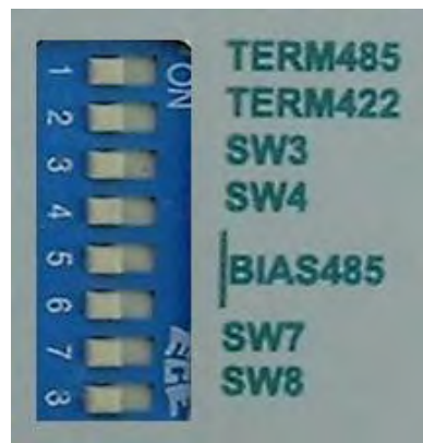
Fig. 7 – Front panel switches, module UC485 (they are all OFF in this figure)
