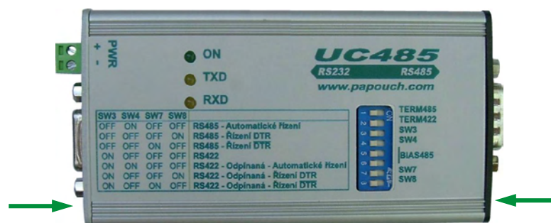
Fig. 9 – Locations of the screws securing the top lid
