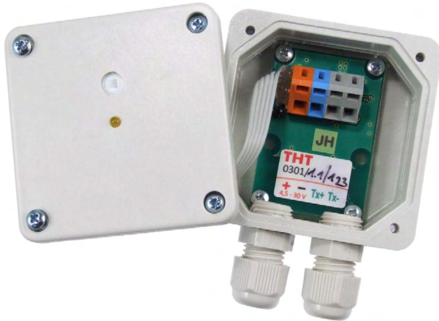
Fig. 5 – Electronics layout inside the box
