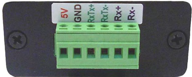
Fig. 1 – Contacts of RS485/422 line connection
