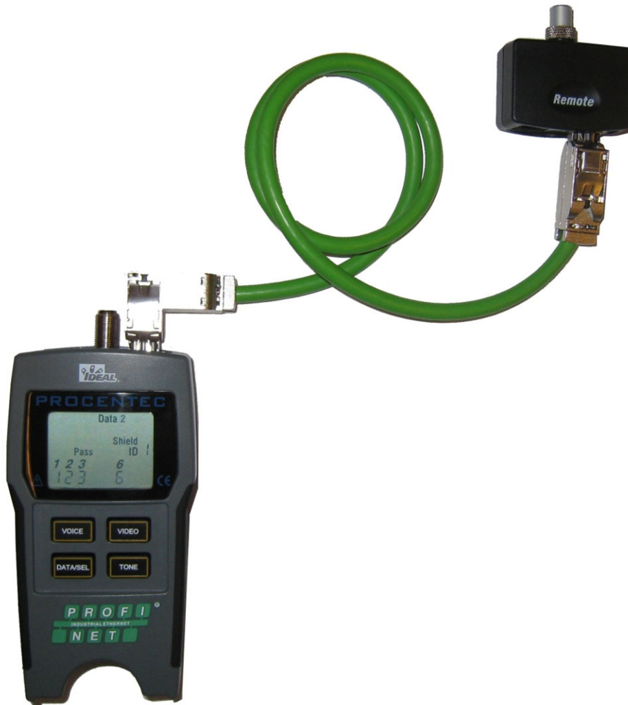
Fig. 4 - Cable attached to the Main and Remote Unit
