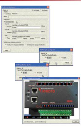
**The Rhio10,** Remote I/O Manager is simple and easy-to-use Ethernet Data Acquisition System that communicates with PCs and other computers over Ethernet and Internet networks. They utilize the open systems environment of Ethernet to acquire data from any number of remote locations.
