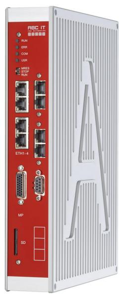
4 Gigabit CPs, 3 fieldbus masters and the unique opportunity to work on S5 and S7 programs simultaneously, the issue of retrofitting SIMATIC S5/S7 systems gives a new dimension.
