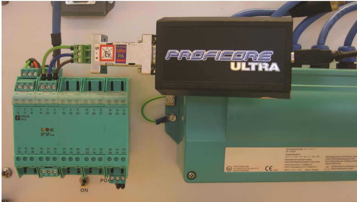
Fig. 12 - Attaching the PA Probe to the installation
