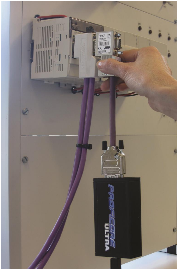
Fig. 10 - Attaching the ProfiCore to a DP installation
