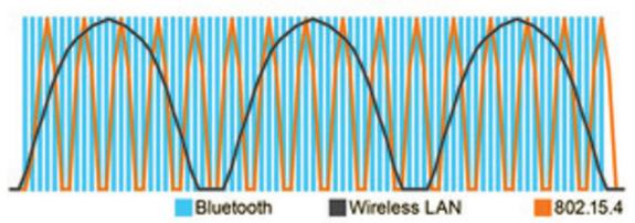
WLAN, Bluetooth and IEEE 802.15.4 work in the same 2.4 GHz frequency band.
