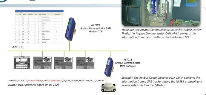
"We found the Anybus Communicator quite easy to use," says Bart de Roo and Steven Lowyck, Control Engineers at APM terminals. "After a three-month test period, we had the first system in place in a straddle carrier which could be monitored from the office. A real advantage of the Anybus Communicator is that the configurations can be re-used. This means that by simply changing addresses, we can immediately apply a new Communicator in another straddle carrier."
