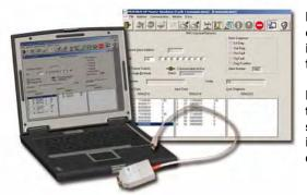
For example, you can use the tool to test the wiring of the inputs and outputs of an I/O block or even read and write analog values. The Master Simulator is useful during setup of the Slave/Adapters in the network as well as during final inspection tests at the device manufacturer.
