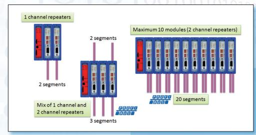
→ COMbricks is based on a backplane into which 10 hot swap repeater modules with 2 channels each can be inserted (20 galvanic isolated transparent segments). Every channel can handle 31 devices and maximum 1200 metres cable length (depends on the baudrate).
